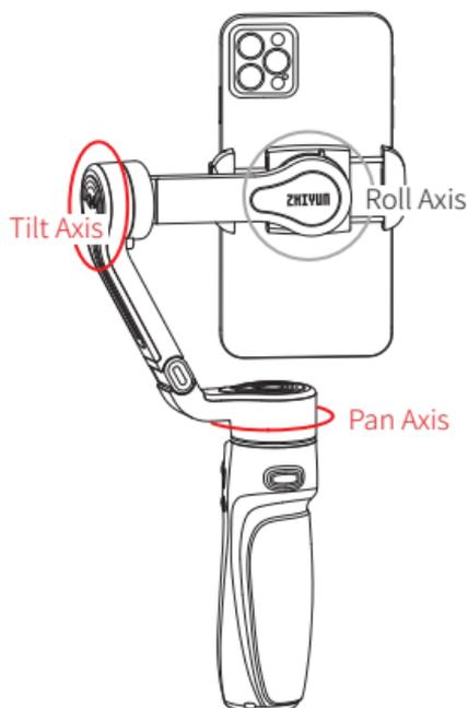
💡 Motors circled in red will follow the movement of the gimbal, while motors circled in grey are locked.
