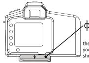
The centering index mark (not on all models) is always laser engraved on the back of the plate. Use this mark to center your camera in the clamp when shooting panoramas.
